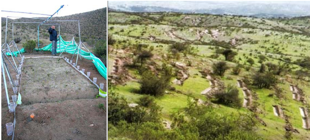
Figure 1. Hillslope with impluvium and infiltration trench in the Elqui Valley (left) and watersheds with (front) and without (back) infiltration trenches in the Metropolitan Region (right)
