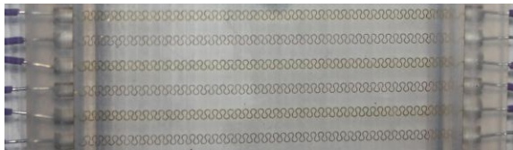
Figure 5: Horseshoe-shaped interconnections embedded into PDMS.
