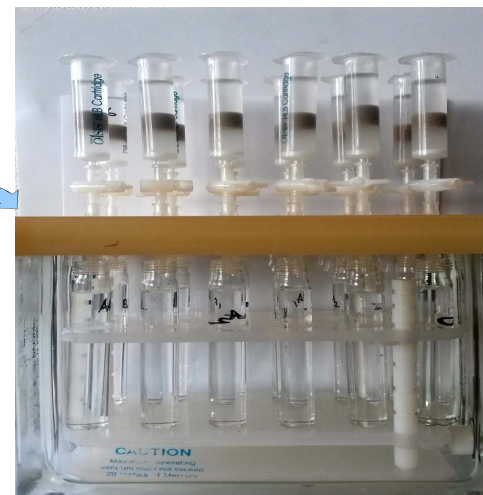
Fig. 2. SPE set up for fractionation of polar fatty acids.
