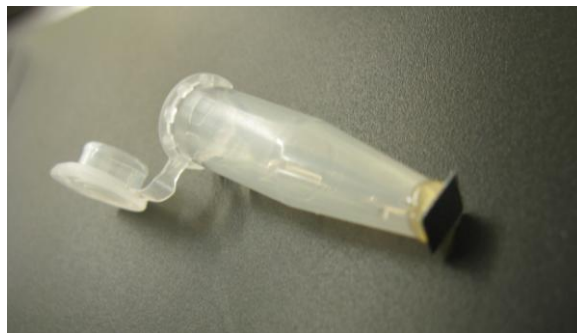
Figure 5. Silicon photonic chip with the array of sensors and the embedded microfluidic system incorporated in the bottom of a reaction tube.
