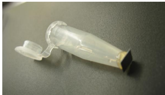
Figure 1. Silicon-on-insulator photonic chip integrated at the bottom of a reaction tube.
