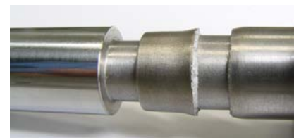
Figure 15: Shearing of tube metal during tensile test
