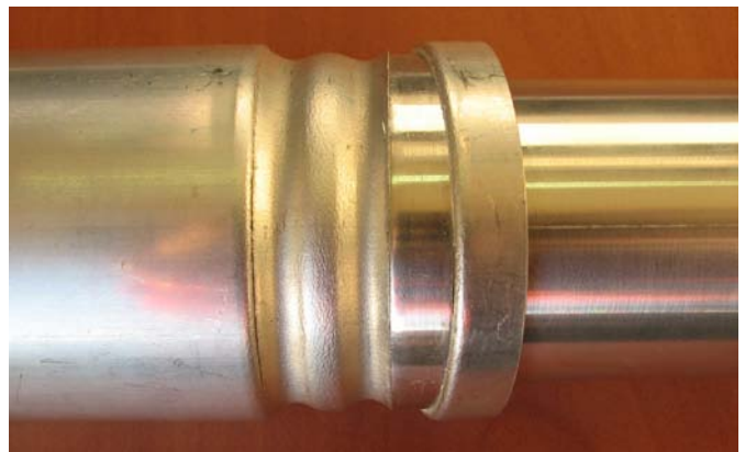
Figure 11: Mandrel with sharp edges cuts the tube
