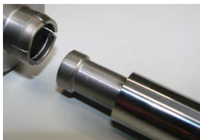
Figure 14: Tube with 4 cracks as a result of radial forces during relative sliding in the tensile test
