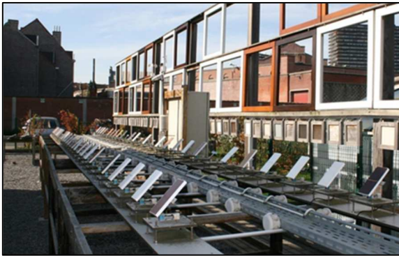
Figure 1: Continuous Moisture Measurement (CMM) set up at UGent – Woodlab
