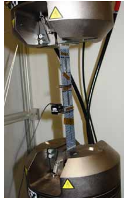
Figure 5. Experimental tensile test set up for measuring the local strains in the composite inner layers using FBGs.
