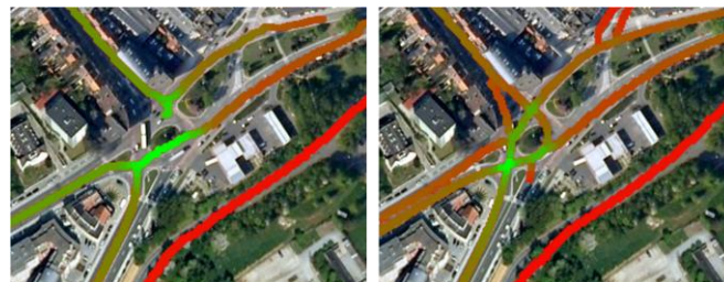
Figure 4. Examples of deriving geometry from gps location data. Left image based on two dimensional rastering: the detailed structure of the roundabout is lost. Right image based on three dimensional rastering: structures are well preserved.
