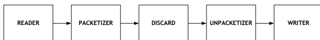
Figure 3: Directed graph configuring the xStreamer as impairment tool which drops parts of frames. The component discard drops the packets it receives with a given probability.
