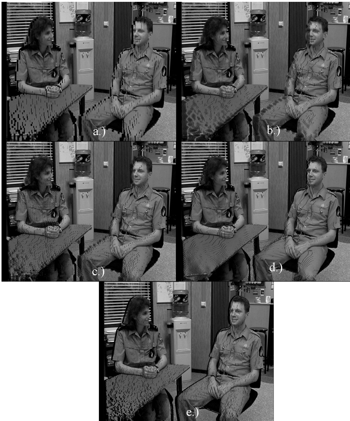
Figure 5. Artificial views generated using a.) Low resolution depth map b.) Depth map obtained by using Lanczos interpolation kernel c.) Depth map obtained using the superresolution method from Farsiu 7 d.) Depth map obtained by superresolution from proposed method e.) Original high resolution depth map
