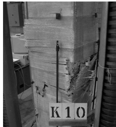
Fig. 2 Confined concrete columns failed by fracture of the FRP after testing.
