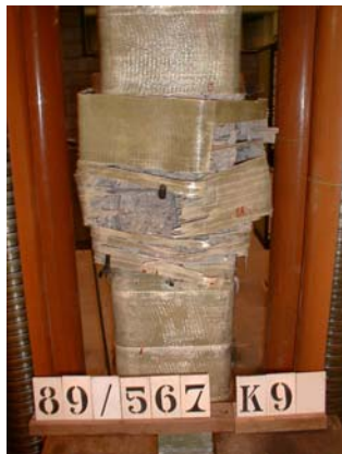
Fig. 2 Confined concrete columns failed by fracture of the FRP after testing.
