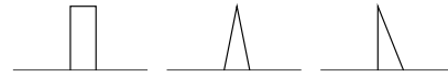
Fig. 6. The three different shapes we examined the robustness with: a rectangle and two triangles as the actual form of the glitch
