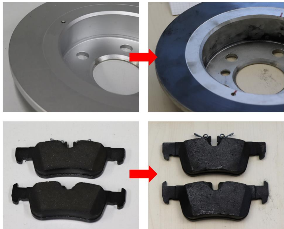
Figure A5. Original brake disc and brake pads of the test vehicle BMW i3 before and after the experiments.
