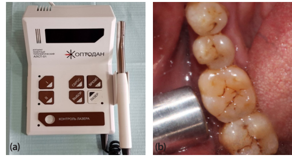
Figure 2. Low-level diode laser "OPTODAN" device (a), Positioning of the laser tip during application (b)
