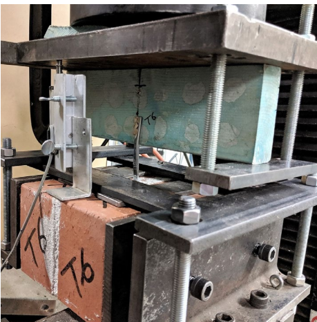
Figure 3. Couplet testing setup for (a) compression and (b) tension loading
