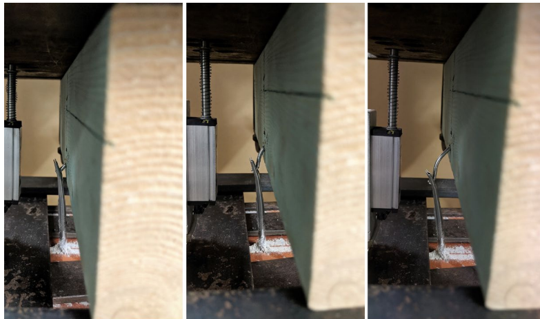
Figure 6. Nail pull-out from timber in tension specimens
