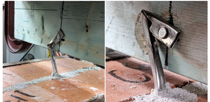
Figure 4. Tie buckling and failure for compression loading
