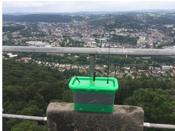
Figure 4.4: Waterproof static sensor box deployed.
