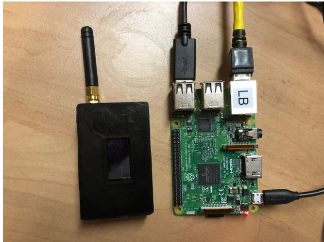
Figure 4.3: BLE LoRa modem with plain Raspberry Pi 3 for size comparison.
