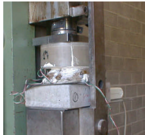
Figure 2. Test setup with claw placed on concrete floor sample
