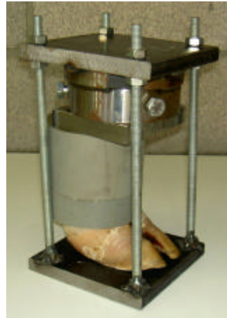
Figure 7. Claw under load in steel frame
