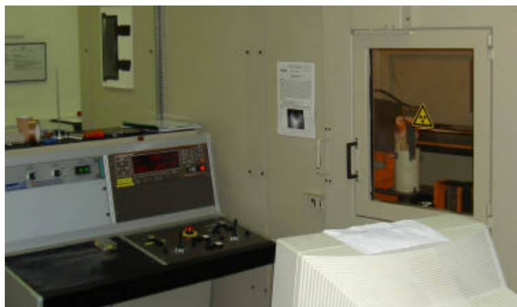
Figure 4. CT scanner with claw placed on turntable behind window
