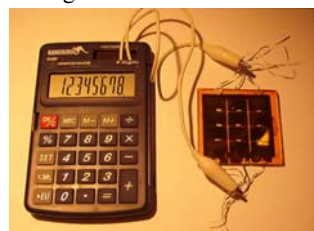
Figure 5: Organic solar cell module with printed active layers driving a small pocket calculator
