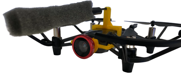
Fig. 2: Tello drone with all accessories mounted.
