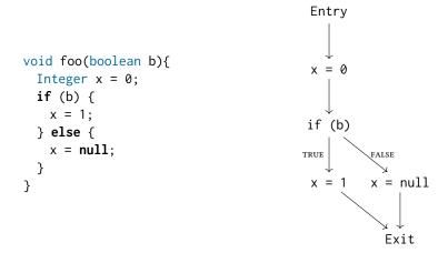
Figure 2: Source level control-flow graph of the foo method, showing the branching behaviour of the if-statement.
