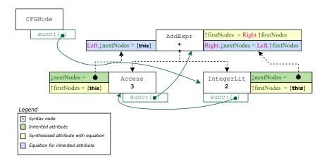
Figure 8: Example of definition of \phextNodes and \taufortimetristNodes for the Teal AddExpr using right-to-left operand evaluation. All the nodes are CFGNodes. Dashed arrows indicates the location of the equation for an inherited attribute.
