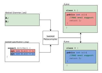
Figure 6: JastAdd generates Java classes from the abstract grammar, and weaves in code corresponding to the intertype declarations in the aspect into the generated classes A and B. Additional RAG code for on-demand evaluation support is elided.
