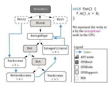
Figure 5: An assignment with a complex left-hand side.
