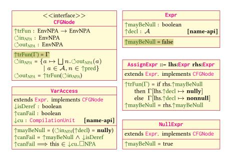
Figure 11: Partial implementation of our NPA. We obtain  $\uparrow$ decl and  $\downarrow$ cu from ExtendJ's name analysis API.
