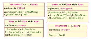
Figure 3: Example application of the IntraCFG framework.
