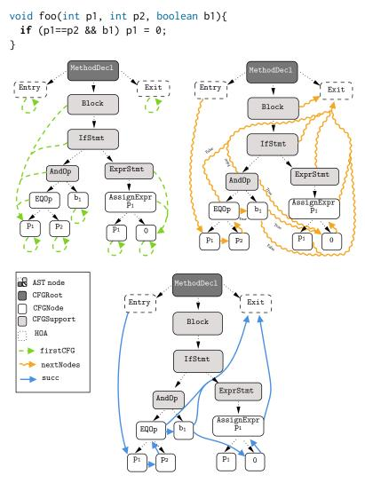
Figure 4: Visualization of the attributes  $\uparrow$  firstNodes,  $\downarrow$  nextNodes and  $\uparrow$  succ. For boolean expressions (AndOp and EQOp), the subsets  $\downarrow$  nextNodesTT and  $\downarrow$  nextNodesFF are shown instead of  $\downarrow$  nextNodes, marked by True and False, respectively.
