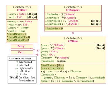
Figure 2: The Intracer framework with interfaces CFGRoot, CFGSupport, CFGNode, and synthetic AST types Entry, Exit. Highlighted attribute equations are default equations, intended for overriding.
