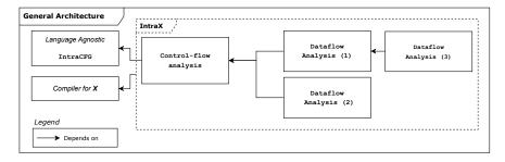
Figure 7: Overall architecture of instantiating INTRACFG for a language X.
