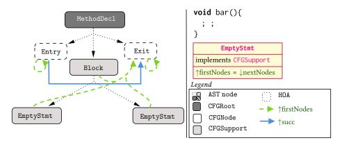
Figure 7: The CFG can entirely skip AST nodes.
