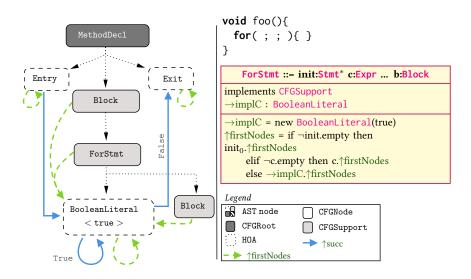
Figure 6: CFG for method with empty *ForStmt*. The HOA  $\rightarrow$ implC reifies the implicit *true* condition.
