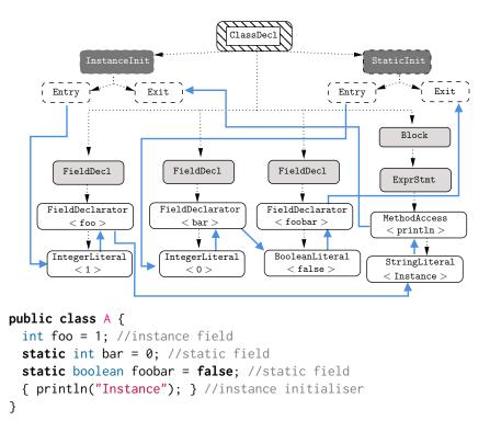
Figure 8: Example of class that interleaves static and instance initialisers. The  $\rightarrow$ instanceInit and  $\rightarrow$ staticInit HOAs represent the CFGs for each kind of initialisers.
