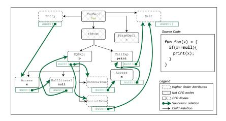
Figure 18: Example of control sensitivity in IntraTeal.
