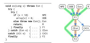
Figure 9: Complex exception flow in a conservative CFG. Only the flow paths in green and orange are realisable.
