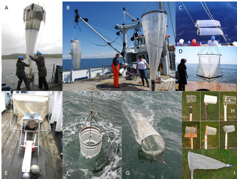
Figure 2.1 Sampling jellyfish with plankton nets: (A) Multinet; (B) CalCOFI net (left) and WP3 net (right); (C) Bongo net; (D) Isaac-kid mid water trawl; (E) video-plankton-net. Difference between vertical tow with WP2 net (F) and oblique haul with CalCOFI net (G). (H) Different versions of 'home-made' devices (© C.E. Mills) for qualitative jellyfish sampling and (I) handheld dip-net
