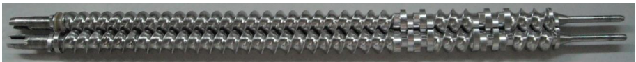
Figure 3.2: Screw configuration with 12 kneading discs (2 blocks containing 6 kneading discs each) indicating the geometry of screws used in a TSG.
