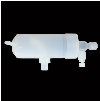
(b) PFA double-pass Scott-type spray chamber. 62
