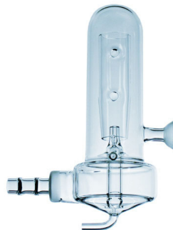
(e) Quartz dual cyclonic/Scott-type spray chamber. 65
