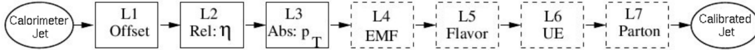
Figure 4.2: Overview of the factorised approach for applying Jet Energy Corrections. The three mandatory first steps are applied in this analysis. They are responsible for rendering the jet energy response uniform across the phase-space covered by the detector [2]. Calorimeter jet technically refers to a jet that has been reconstructed using calorimeter but also tracker information.
