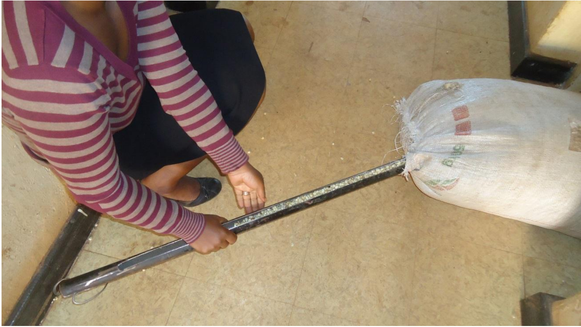
Annex I: An improvised sampling spear used to draw samples discussed in Chapter 2.
