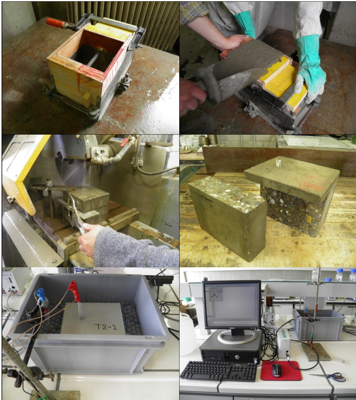
Figure 9.2. Sample geometry and experimental setup for monitoring of the corrosion potential of a rebar embedded in concrete versus a SCE reference electrode.
