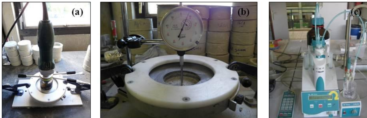
Figure 6.2. Test setups for profile grinding (a) and grinding depth measurements (b) and the Metrohm MET 702 automatic titration apparatus (c).
