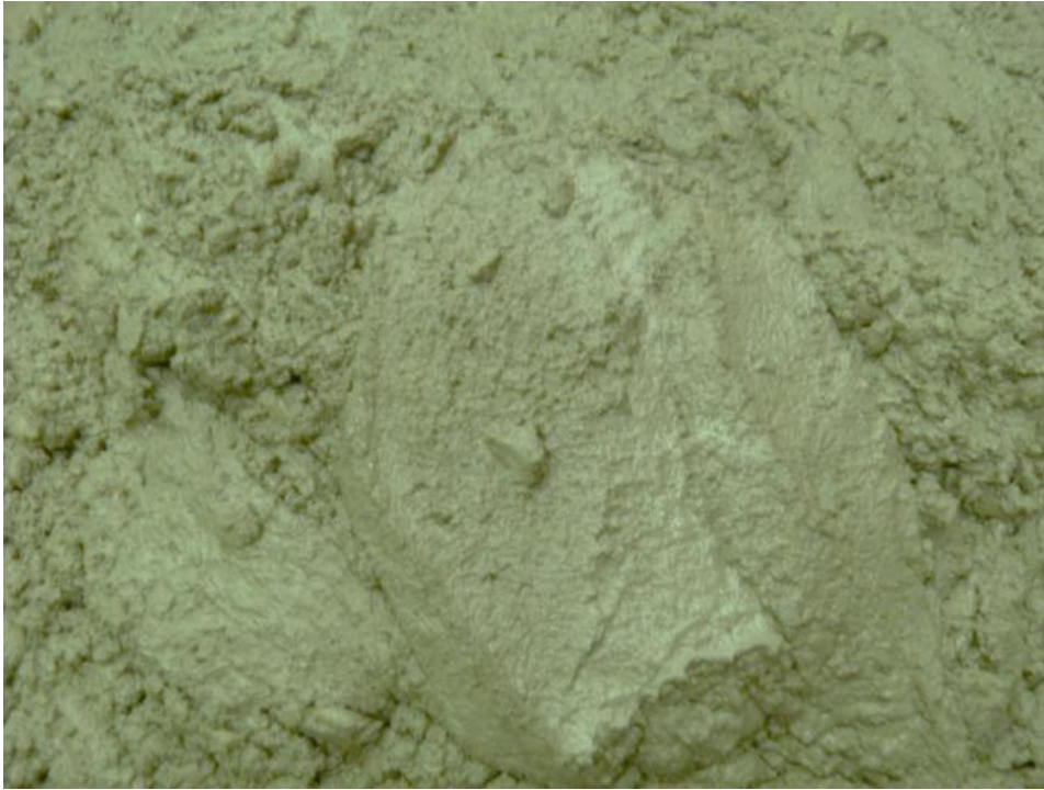
Figure 7.13. Influence of additional intermittent mixing on the fresh state appearance of air entrained FA+SF concrete.
