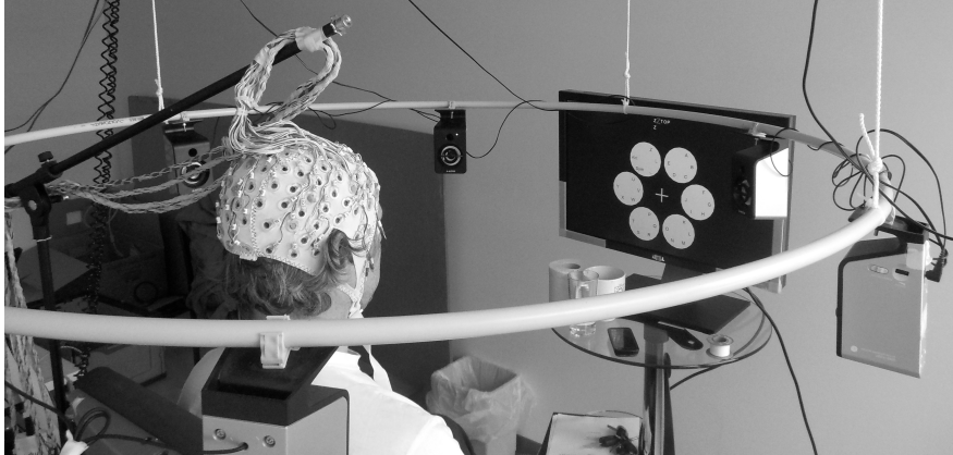
Figure 1.5: The AMUSE spatial auditory ERP setup. The user sits in the centre of a ring, on which 6 speakers are positioned. A specific tone is associated with each of the 6 speakers. By attending one of the six stimuli, the user can perform an action. This picture was taken at the TU-Berlin during the pilot study for the evaluation of the unsupervised algorithm that is proposed in this thesis. The eagle-eyed readers can spot a NIPS mug, which is a much needed accessory in a machine learning lab.
