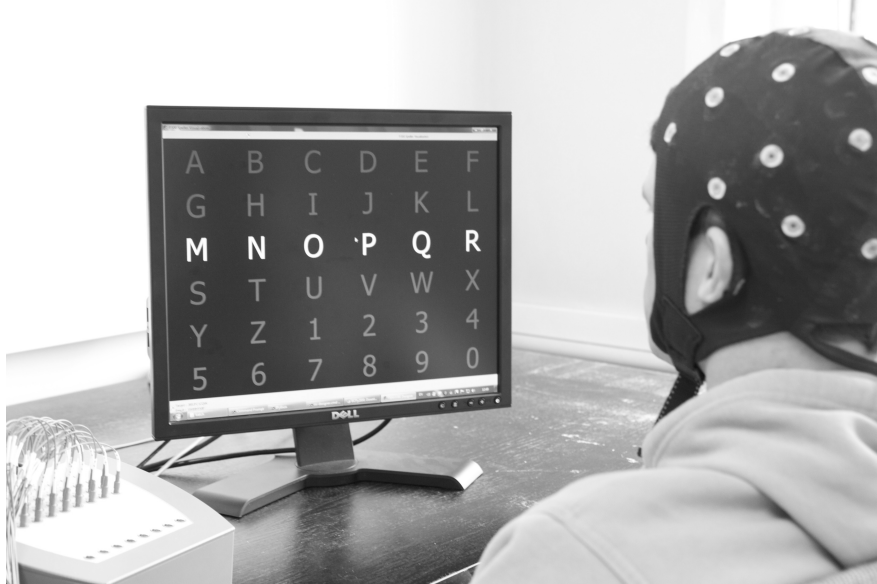
Figure 1.4: An experimental setup for visual ERP spelling. (photo: Francis wyffels)
