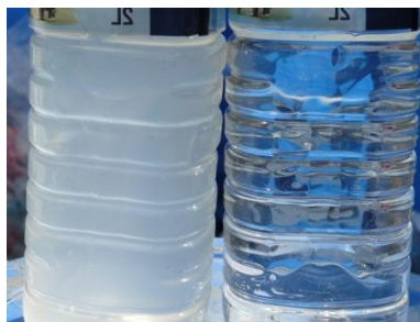
Figure 4.8: Picture of the shower wastewater before (left) and after filtration (right).
