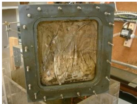
Figure 3.8: semi-dead-end membrane module used in this chapter 4 (and with support in chapter 5).
