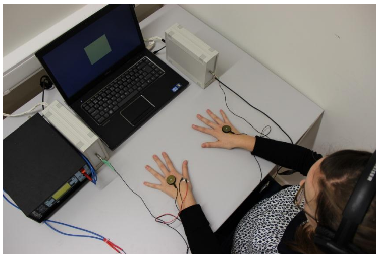
Figure 4. Example of experimental setup. Tactors (large round circles) were placed on both hands. Electrodes for painful stimulation were placed on one hand. In order to induce threat, colored cues were used that signaled whether or not a painful stimulus could be administered.
