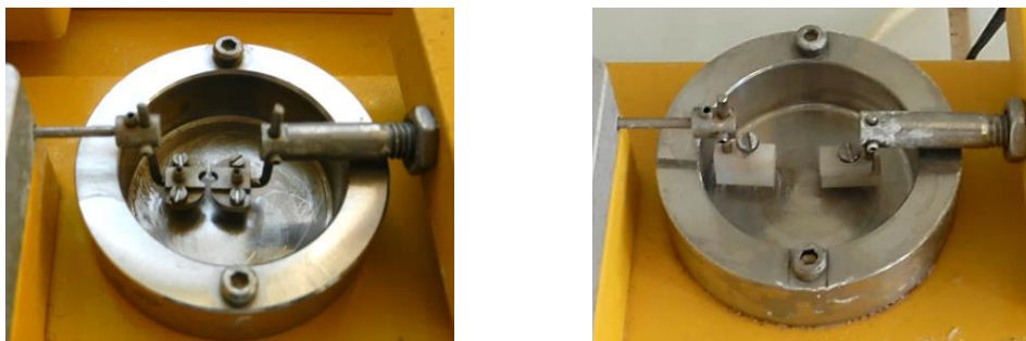
Figure III.4: Organ bath with half-moon shaped holders for mounting arterial ring segments (left) and holders for clamping CC strips (right).
