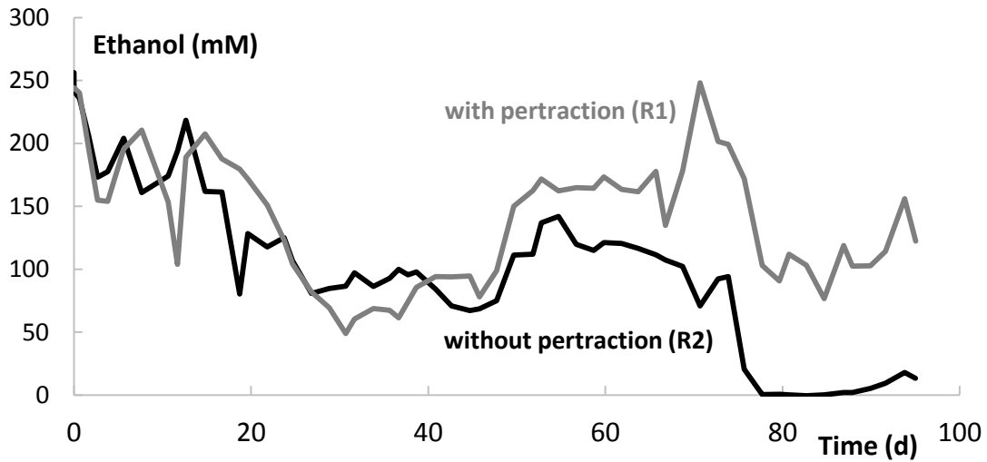
Figure App. 4.6 - Ethanol concentration in the reactor broth, for both bioreactors.
