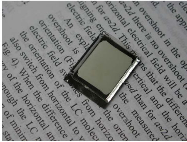
Fig. 1.4: Due to the light scattering this reflective PNLC display has the same appearance as white paper.
