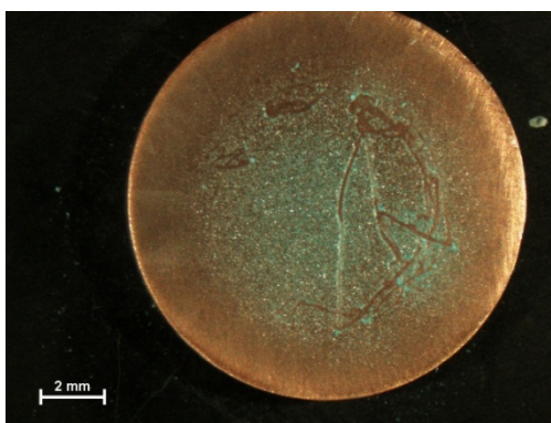
Figure 6.5: Optical micrograph of a copper coupon treated for 24 h in a 0.1 M \text{HC}_{12} ethanolic solution.
