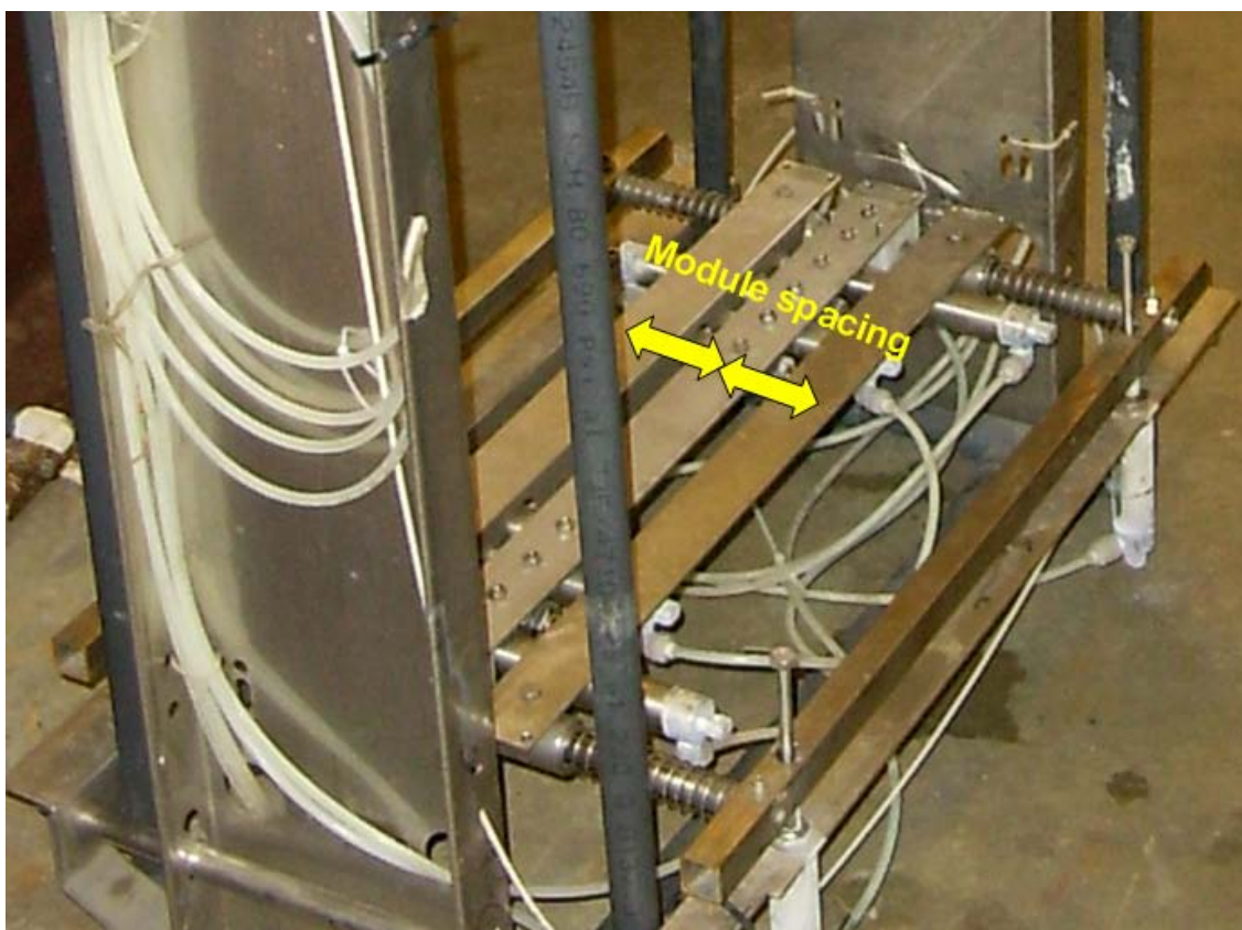
Figure 8.2. Spacing between the three modules
