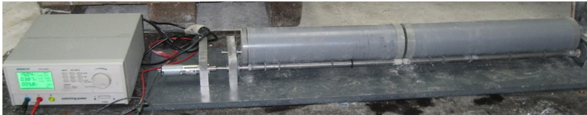
Figure 4.6. Rotation machine to prevent segregation
