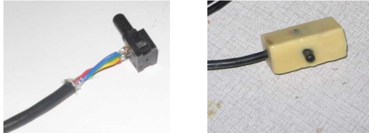
Figure B.2: Detail of 'naked' pressure gauge (left) and gauge covered with epoxy coating (right).
