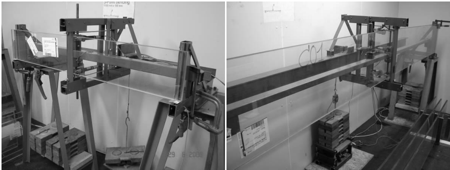
Figure III.30: Bending test setup with specimen placed vertically: small creep experiment for test samples B and E with a span of 1050 mm (left); large relaxation experiment for test samples C with a span of 2950 mm (right)
