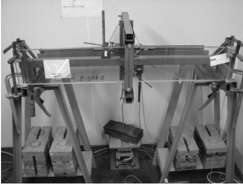
Figure B.6: Small bending creep test on test specimen B14
