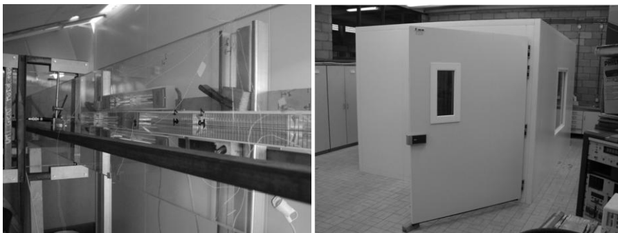
Figure III.14: Bending experiment with IR-heaters (left); chamber with temperature and humidity controlled environment (right)
