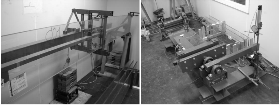
Figure B.7: Large bending relaxation test on specimen C01 (left); Torsion relaxation test setup with specimen D01 (right)
