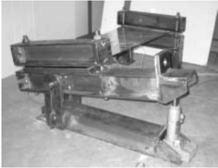
Figure III.12: Torsion test setup and results of glass/PVB laminates by Kasper [Kasper 2005]
