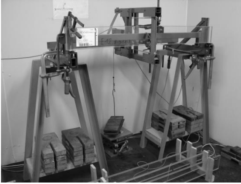
Figure A.8: Small bending creep test on test specimen E12
