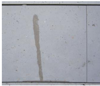
Figure 9. Micro runoff test.
