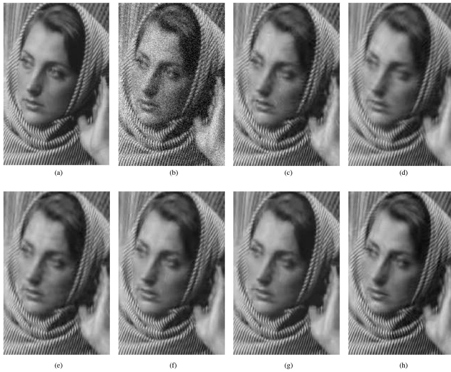
Figure 3.9: Detail of the denoising results of Barbara . (a) the original image, (b) the noisy image (noise standard deviation 20), denoising result of (c) ProbShrink , (d) curvelet hard thresholding, (e) BiShrink , (f) BLS-GSM , (g) BM3D and (h) ProbShrinkCurv .
