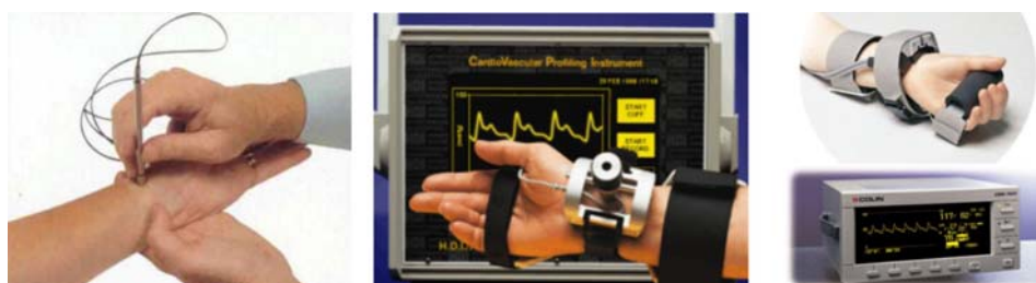
Figure 2–8 Current commercially available tonometers: Millar ® Instruments pen-probe (left), Hypertension Diagnostics ™ wrist-probe (middle), Colin ® Medical Instruments Corp. automated probe (right).
