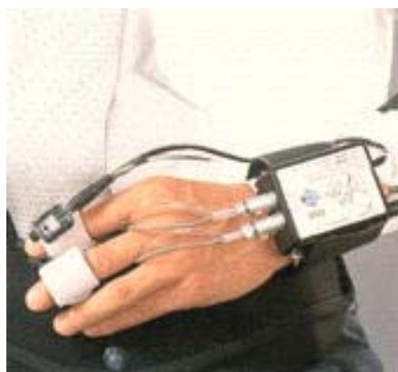
Figure 1–6 Measuring finger arterial waveforms with the Penaz method (Finapres ® device, FMS Finapres Medical Systems, Arnhem, NL).
