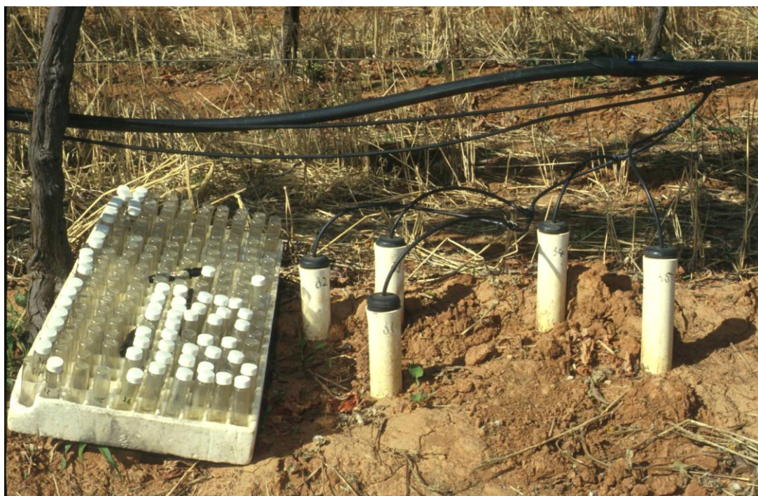
Figure 4.03 The positioning of 5 suction cup lysimeters (5 depth increments) between two vines with a cartridge of empty bottles on the left.
