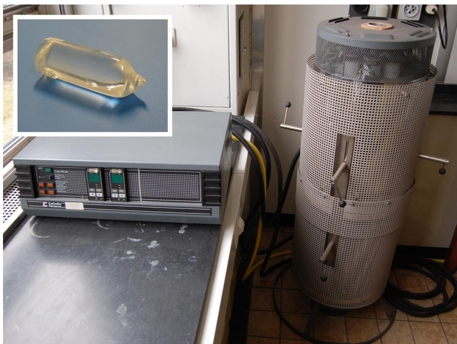
Figure 3.13. Bridgman setup with two furnaces at constant temperature. The inset shows an undoped Bridgman grown CsBr single crystal.
