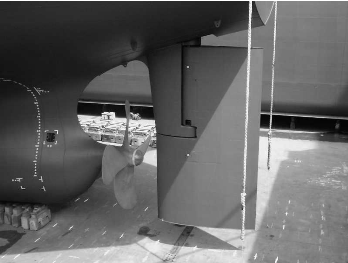
Figure 1.6 Three interacting modules of a ship: hull, propeller and rudder
