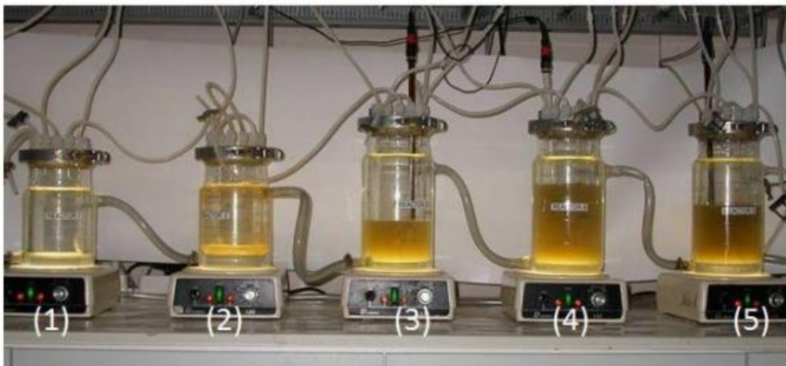
Figure 30. SHIME reactor. 1) stomach, 2) small intestine, 3) ascending colon, 4) transverse colon, 5) descending colon
