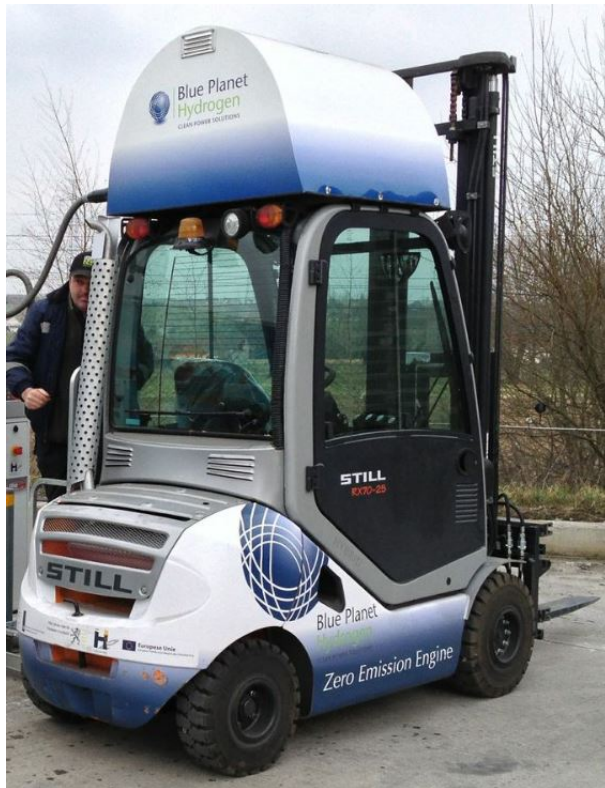
Figure 2: Forklift truck equipped with a H 2 ICE, part of the demonstration activities within the Hydrogen Region Flanders - South-Netherlands project [21]
