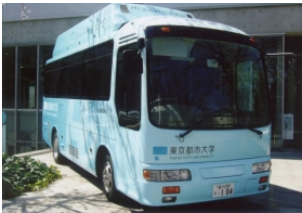
Figure 4: Microbus equipped with a 4.7L 105kW hydrogen engine, demonstrated by Tokyo City University [3]. Permission to reproduce granted by copyright holder Tokyo City University.
