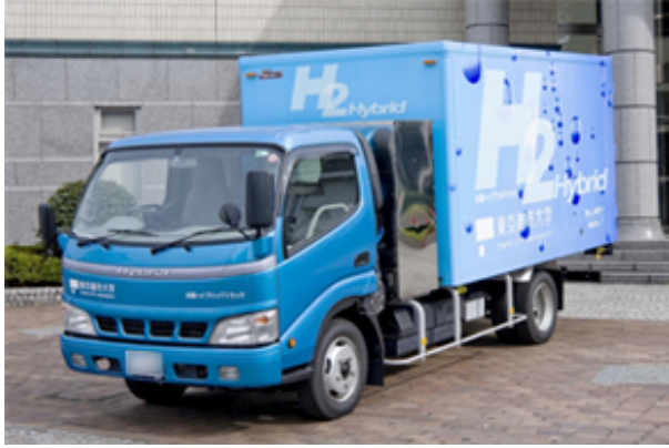
Figure 3: Hybrid light duty truck equipped with a 4L 91kW hydrogen engine, demonstrated by Tokyo City University [3]. Permission to reproduce granted by copyright holder Tokyo City University.
