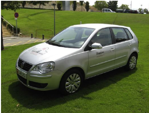
Figure 1: Bi-fuel (gasoline/hydrogen) VW Polo demonstrated by the University of Navarre [5]. Permission to reproduce requested.
