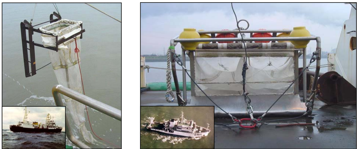
Figure 10.2. The hyperbenthic sledges used for the sampling of mysid shrimp in the Scheldt estuary. Left: the sledge operated from the RV 'Zeeleeuw' (inlay) during the first 5 campaigns (March-June-November 2001, March-June 2002). Right: the sledge operated from the RV 'Belgica' (inlay) during the last 2 campaigns (December 2002 and March 2003).
