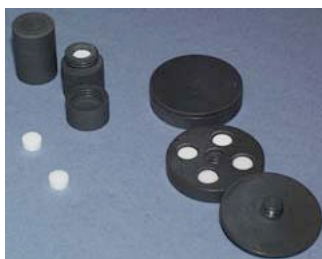
Figure 5.1: An example of an alanine dosimeter system (here in the form of pellets), as supplied by the National Physics Laboratory ( http://www.npl.co.uk ).
