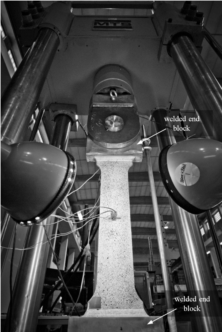
Figure 2.9. MWP specimen mounted in Laboratory Soete's 2500 kN tensile test rig
