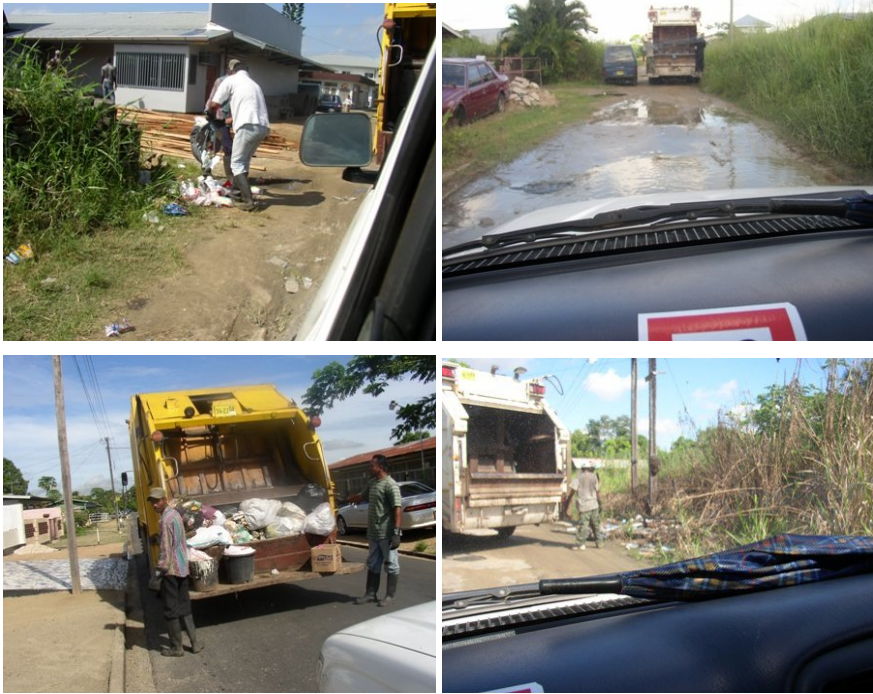
Photo 4.2: Problems during waste collection: burst of plastic bags, condition of roads, compaction of waste in front of residences (leachate from waste and malodors), cleaning of waste collection points
