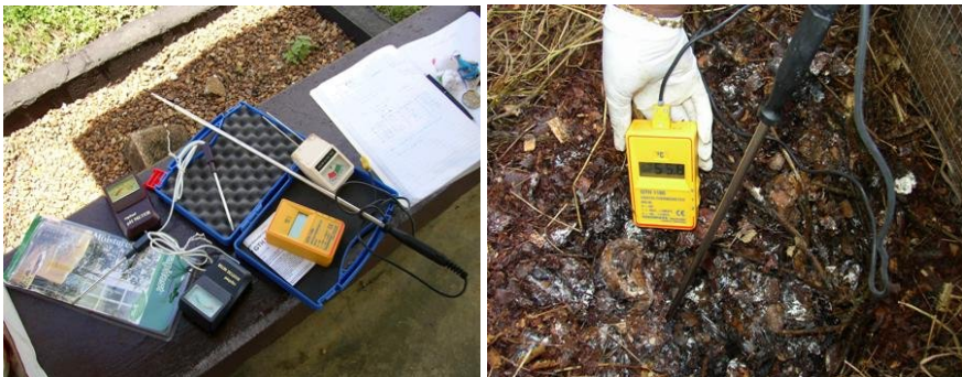
Photo 6.3: Measuring equipment used during composting process
